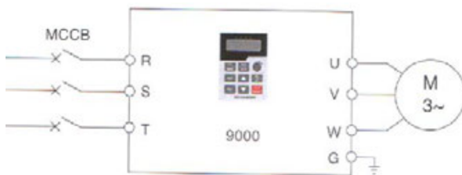
Simple Operating Connection
